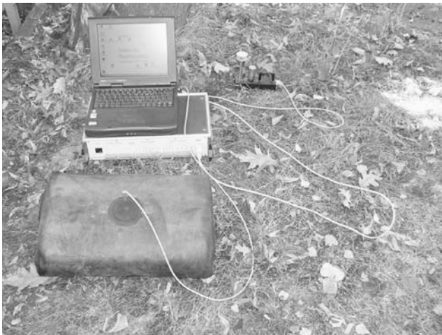
Fig. 1 Dummy A with inserted temperature probe and computerised measurement
